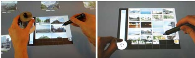
Figure 3: A 3D vs. a 2D handle used in the PhotoLens UI [20].
