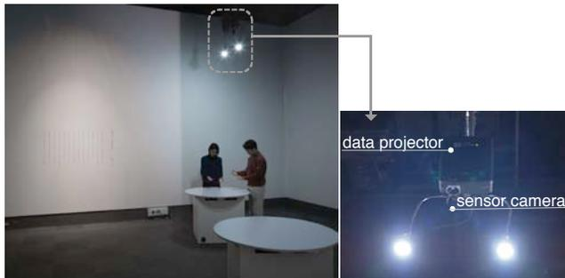
Figure 2. System Structure.
